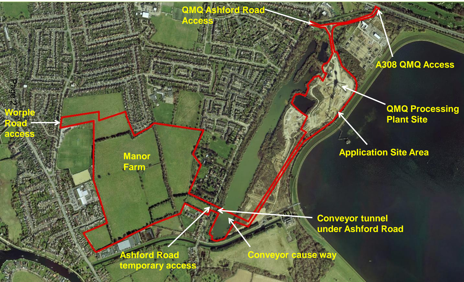
Aerial 2 : Manor Farm and Queen Mary Quarry (QMQ)
